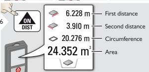
The result is shown in the main line and the measured value above.
