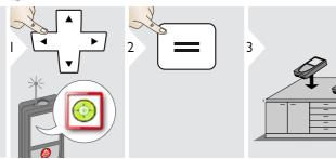
Displays inclinations of 360° with a transverse inclination of +/- 10°. Instrument beeps at 0° and 90°. Ideal for horizontal or vertical adjustments.
