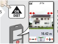
Select arrows with the cursor keys or by tapping on the display and adjust with softkeys. Corresponding width is calculated.
