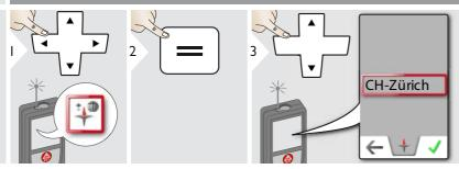
Select the nearest location and the device adjusts the declination accordingly.
