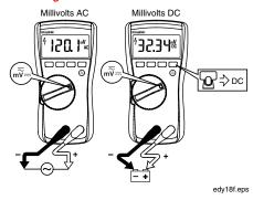
With the function switch in the  $\overline{\mathbf{n}}$  position, the Meter measures ac plus dc millivolts. Press to switch the Meter to dc millivolts.
