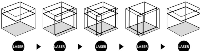
**!** The transport restraint must be released for horizontal and vertical levelling. The laser lines flash as soon as the device is outside the automatic levelling range of 3.5°. Position the device such that it is within the levelling range. The laser lines stop flashing (steady light).
